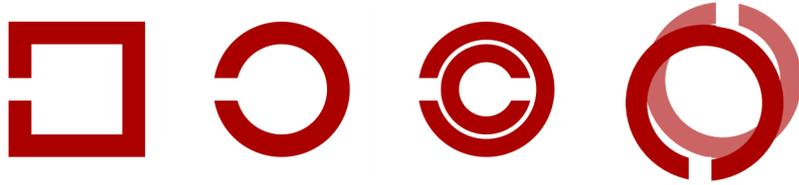
Figure 2.16.: *Rectangular SRR, circular SRR, nested SRR (Double split ring resonators (DSRR)), SRR back-to-back configuration.* [99]
